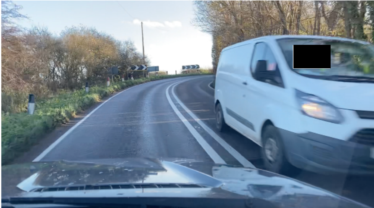
Figure S3: Eastbound uphill approach towards the same bend, demonstrating restricted forward visibility from both directions and limited carriageway width for passing vehicles.
